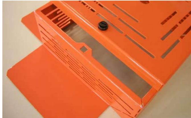
The lid connects by first locating the hinge tabs to the corresponding slots in the chamber body. The lid is secured by a quarter turn of the 'quick lock'. This can be done manually, but a small coin or screw driver will be required to open the lock to gain access to the chamber.
